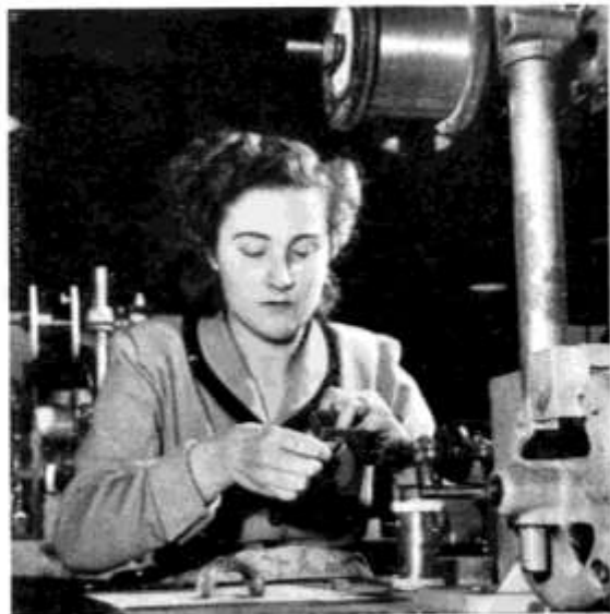
Mrs. Brenda Harrington winding a section of a deflection coil assembly
