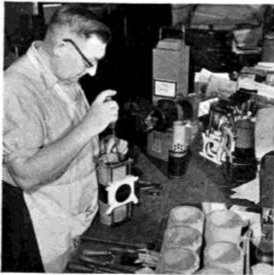
F. Harbridge, Section 21, assembling an Image Orthicon deflection yoke for the Mark II camera
