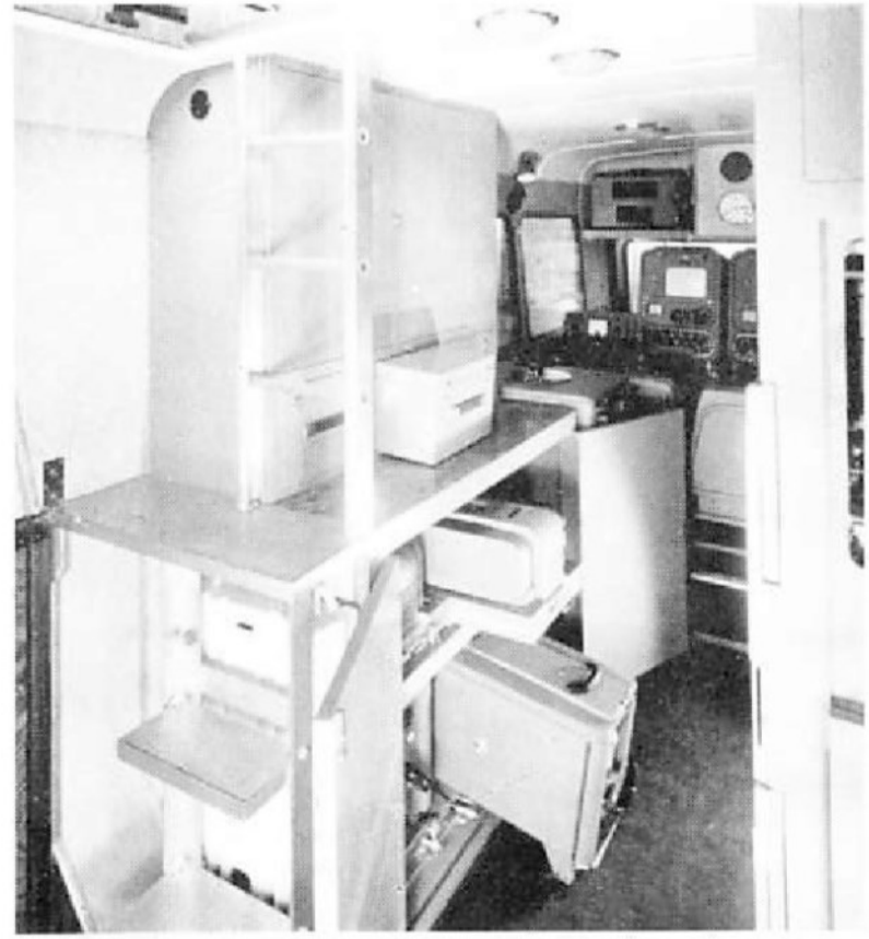
Interior view of one of the two television outside broadcasting vehicles for Canada, showing roof ladder, cameras and view finders in their store cupboards, lens boxes, and tool storage. Another view showing the main desk, broadcast distribution box, three camera control monitors, master control monitor. Above can be seen the sound receiver and "on the air" vision receiver, and on the right the producer's desk.
