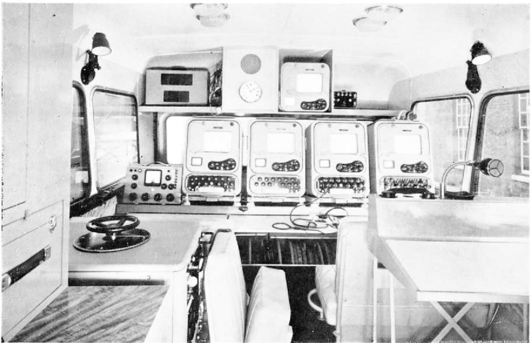
Interior view of one of the two television outside broadcasting vehicles for Canada, showing roof ladder, cameras and view finders in their store cupboards, lens boxes, and tool storage. Another view showing the main desk, broadcast distribution box, three camera control monitors, master control monitor. Above can be seen the sound receiver and "on the air" vision receiver, and on the right the producer's desk.
