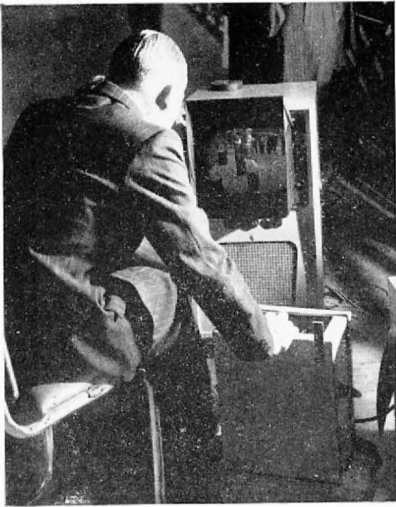
At the Mechanical Handling Exhibition at Olympia in June, an operator remote controls the gantry crane by radio transmitter . . .
