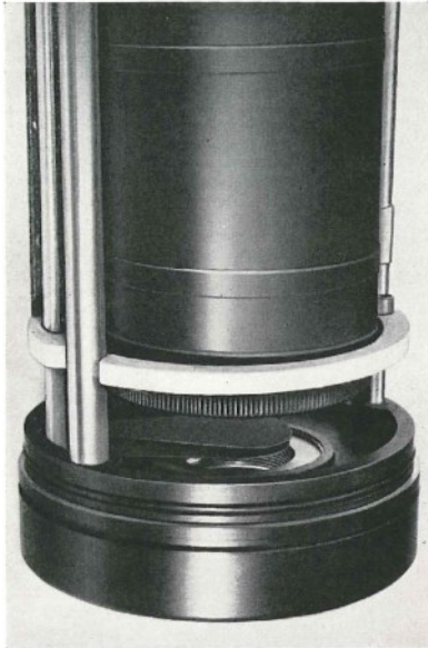
Camera front showing the V 4033 Sun Shutter.
