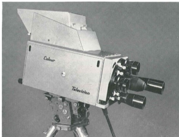
The camera, fitted with viewfinder.
