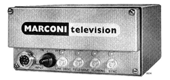
THIS unit is designed for use in industrial installations needing an accurately interlaced picture. It provides separate outputs of line drive, field drive, blanking and mixed synchronizing pulses at an amplitude of 2 volts p-p into an impedance of 75 ohms. The outputs are available on 405, 525 and 625-line systems, but no equalizing pulses are provided.
