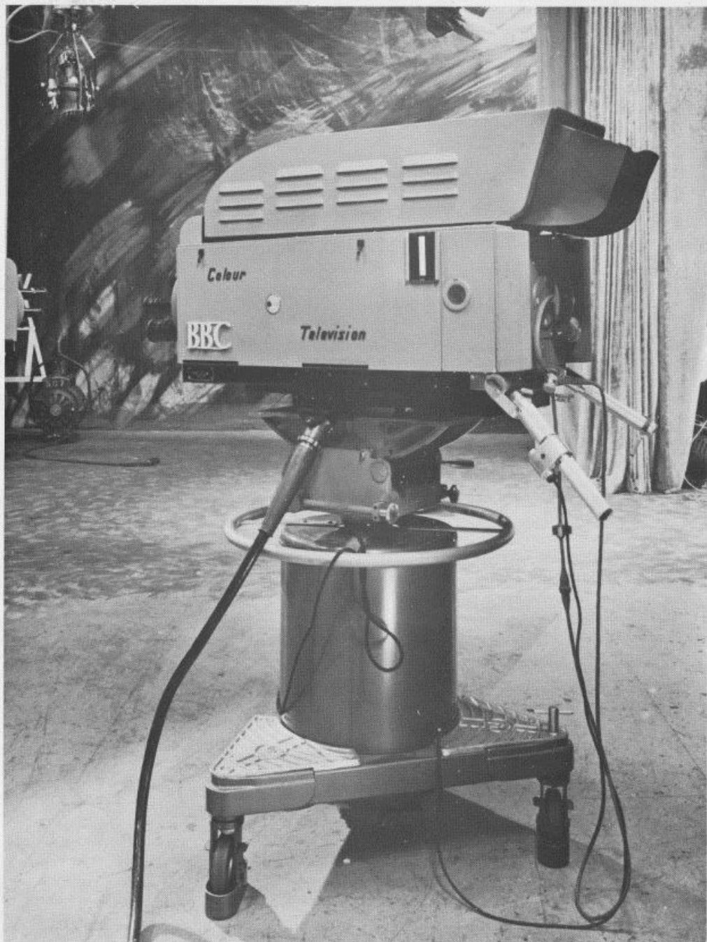
COLOUR CAMERA MOUNTED ON STUDIO CAMERA PEDESTAL
