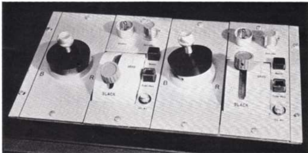
Two Colour Balance Control Panels and two Operational Control Panels mounted in a desk.
