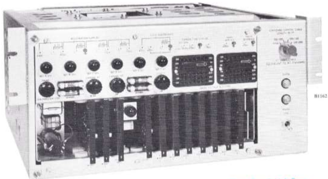
Power Supply Unit, Type B3210, with front cover removed
