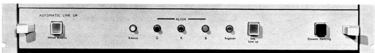
Fig.5 The CCU showing the Automatic Line Up controls.
