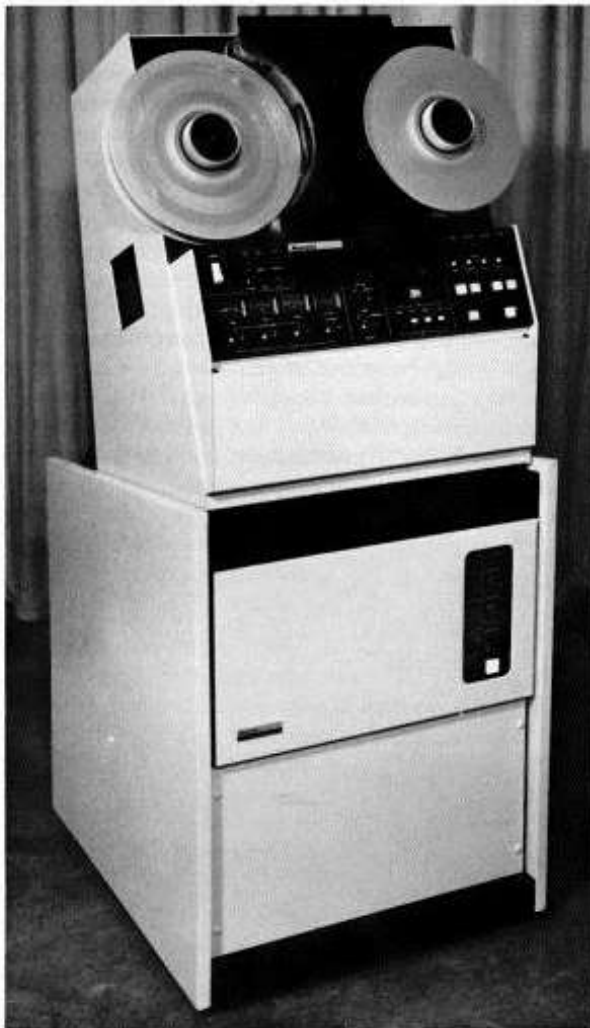
Figure 1. The Marconi MR1 non-segmented helical video tape recorder, with the MTBC1 time base corrector fitted beneath
