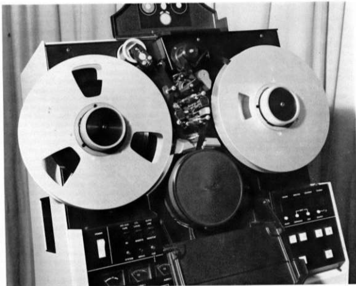
Figure 2. Transport deck of the MR1 video tape recorder
