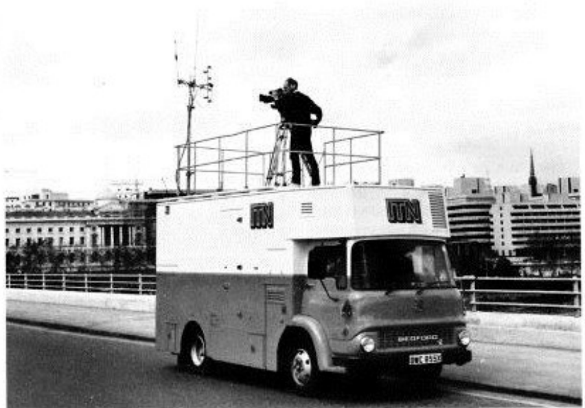
Fig.2. O.B vehicle in use. Antennas for local site communications, talkback and off-air reception can be seen on the partially raised mast at the rear of the vehicle
