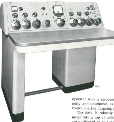
THE CONTINUITY CONTROL DESK Type BD 521 is designed to provide continuity of broadcast programme at controlled level, from a number of studios and outside broadcast sources.
