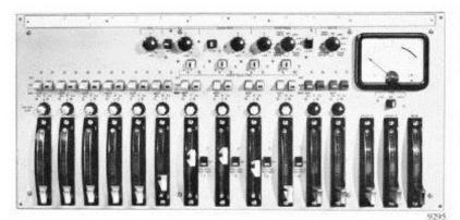
THE BD972 Sound Mixer has been designed for television outside-broadcast units and small television studios. It is mounted in a box, but the front panel and rear connector block can easily be removed for mounting in the customer's own desk. The mixer is fully transistorized.
