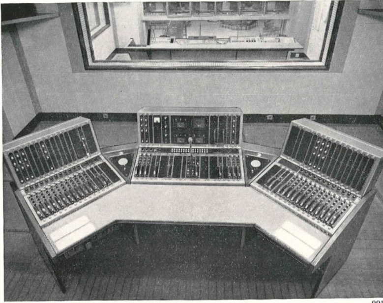
A new transistorized sound control desk installed at Granada Television Centre's Studio 12, Manchester, England.
