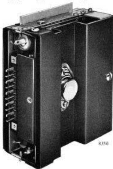
The plug-in amplifier unit of the Type BD 887.
