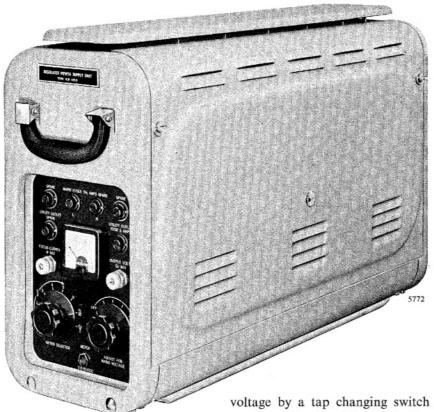
DESIGNED TO SUPPLY both AC and DC power to a camera channel or vision mixer, the Type BD 629 Supply Unit is suited to a variety of mobile applications when a relatively large regulated anode current is required.
