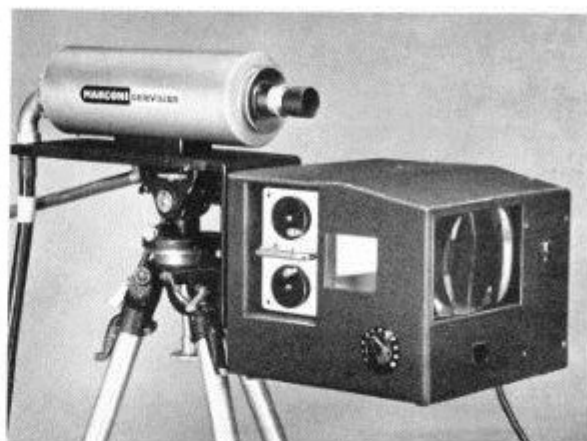
A Type V3020 Vidicon Camera with 'Minicue' attachment. 8401
