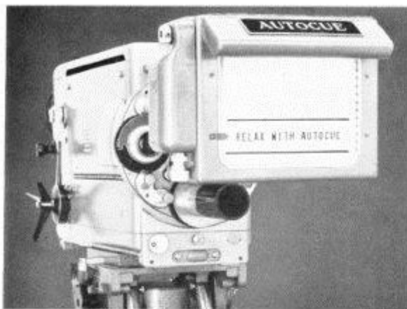
A Mark IV Image-orthicon Camera with 'Autocue' attachment. 8161
