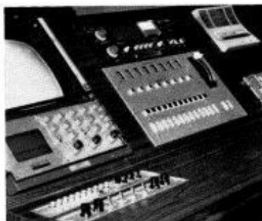
Semi-automatic master switcher at Amman studios of Jordan TV
