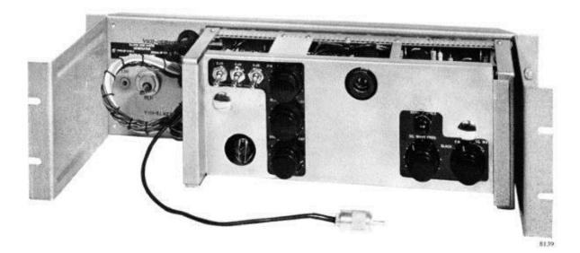
THIS UNIT produces a waveform for testing the transient response of television equipment at low frequencies. The output signal corresponds to the C.M.T.T. Test Signal No. 1. Type 3391 is built on a 19-inch (48 cm) recessed chassis suitable for rackcabinet mounting.
