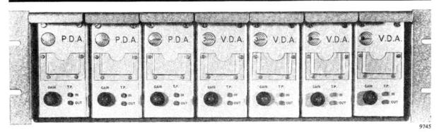
THESE self-contained, fully transistorized amplifiers are module-type units. Up to 35 vision outputs or 42 pulse outputs are available in  $5\frac{1}{4}$  in. (13·3 cm) of a 19 in. (48 cm) rack. A pre-set gain control and output-level test points are provided on the front panel of each module.
