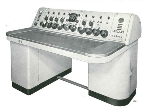
THE TYPE BD 514 Studio Control Desk, which is completely self-contained, provides an extremely flexible high-quality control of programme material from five studio microphones, an announcer's microphone, and from any one of four outside broadcast lines or other high-level sources.
