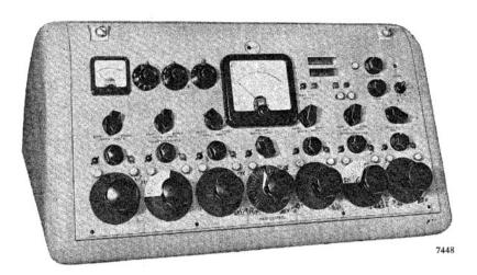
sound control console Type BD 595 fulfils all the requirements of a modern sound studio control position. The facility of operation which is essential in a precision-timed broadcast production is provided by a clear and simple signalling system and a self-evident set of convenientlyplanned controls. Furthermore the needs of a studio system of moderate size are adequately met in a unit of small dimensions which can be integrated with new or existing arrangements.
