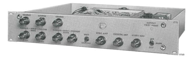
THIS fully transistorized generator replaces the valved BD 959 for operation on 625 and other line standards and produces a signal suitable for testing the linearity of television display units, monitors and receivers.
