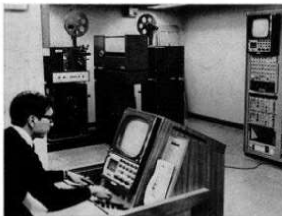
2 Full Facilities Colour Telecine installed by Cable and Wireless at Hong Kong for use in conjunction with satellite ground stations
