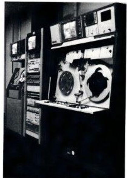
View of the B3410 Telecine and MR2B Video Tape Recorder installation recently supplied to Filmatic Laboratories, a leading specialist film-processing company.
