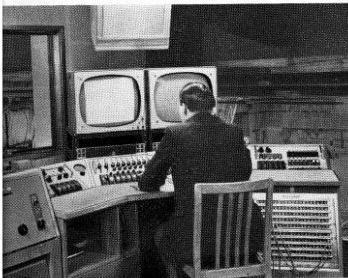
The Sound Control Room. The Disc reproducing desk is seen on the left of the sound supervisor's position.
