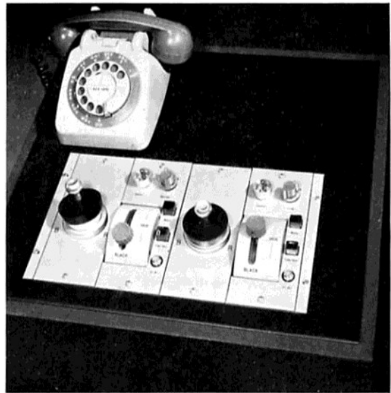
Fig.2 Colour Balance Control Units and Operational Control Panels for Mark VII cameras.
