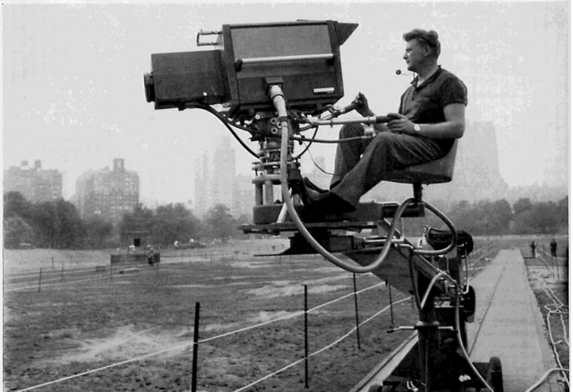
Fig.3 A Mark VII camera on a typical outside broadcast.
