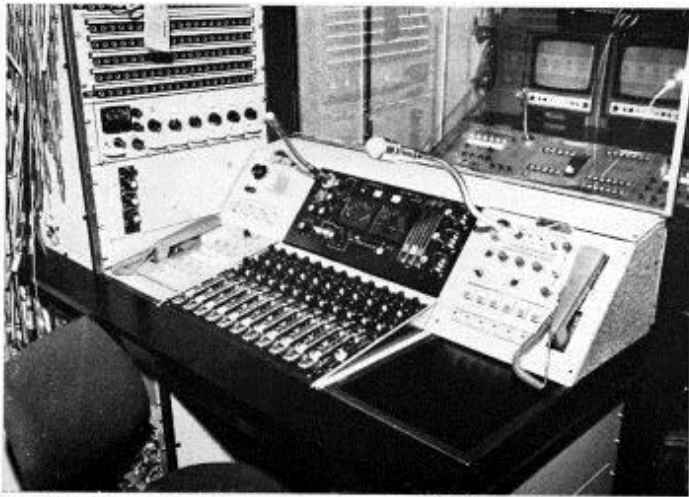
Fig.4 Sound engineer's position showing 12-channel mixing console. (BBC photograph.)
