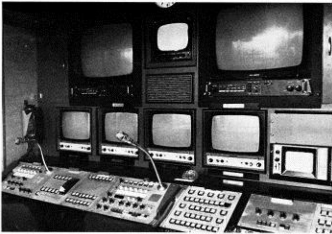
Fig.5 Monitors and control desk with positions for (left to right) vision mixer/production assistant, engineering manager, vision engineer. (BBC photograph.)
