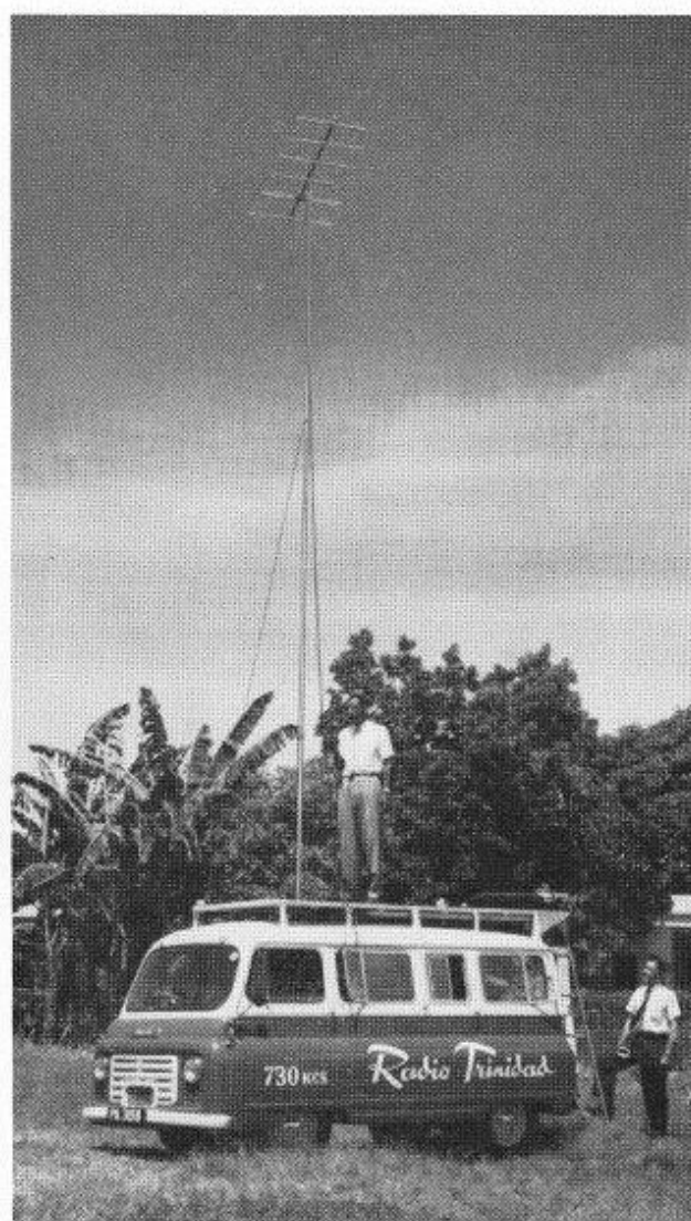
The O.B. van with the aerial erected. The van can move at slow speeds with the aerial in this position.
