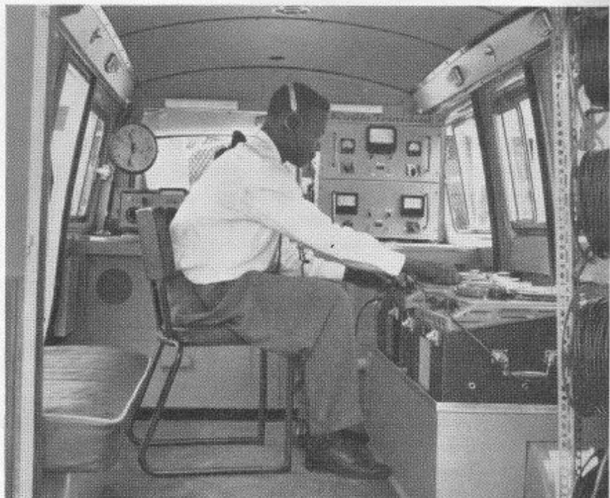
The interior of the O.B van. The neat, compact layout is clearly shown. The accessibility of the equipment is also evident.
