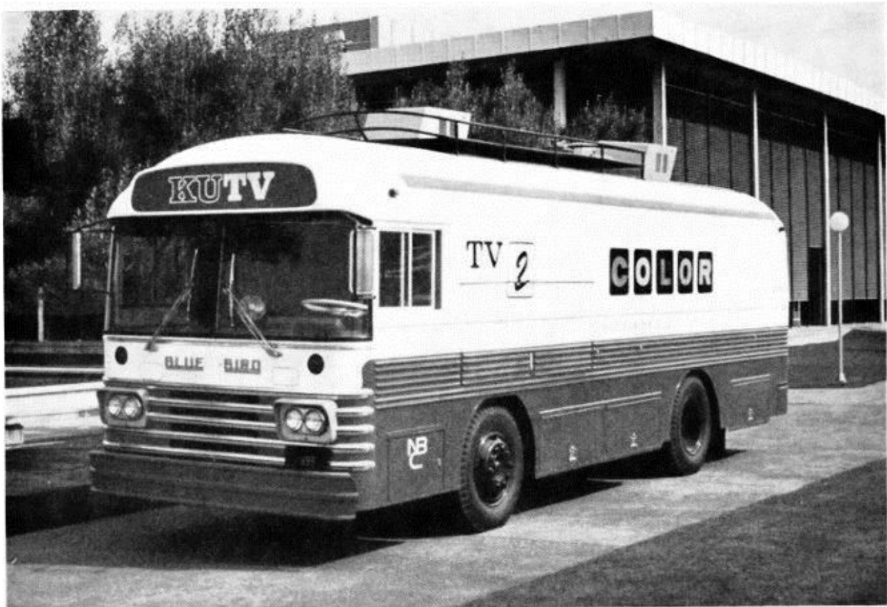
Fig. 2. This versatile colour mobile uses a combination of one or two video-tape recorders and two, three or four Mark VII cameras.
