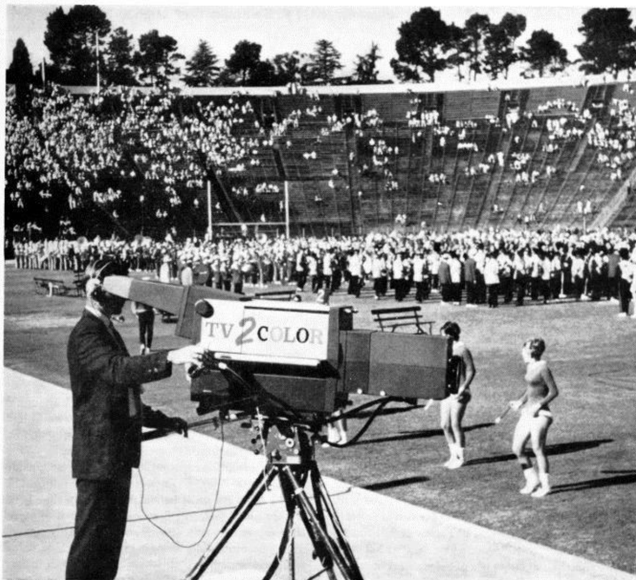
Fig. 1. One of the four Mark VII colour cameras used by KUTV to cover the Stanford versus Washington State ball game.
