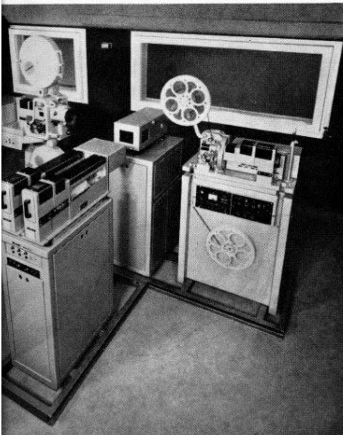
Fig. 3. View of Multiplexer Projector System.
