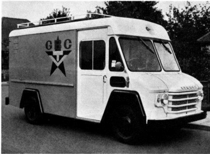
Fig. 1. The two-camera Outside Broadcast Vehicle.
