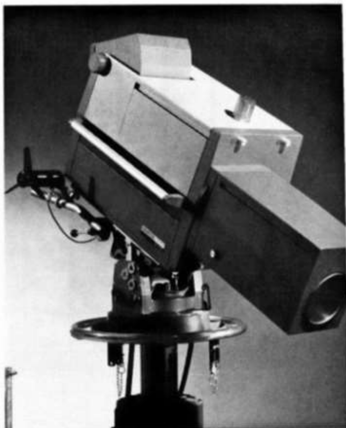
Fig. 1. The Mark VII colour camera using four photoconductive tubes in a Y.R.G.B. arrangement.
