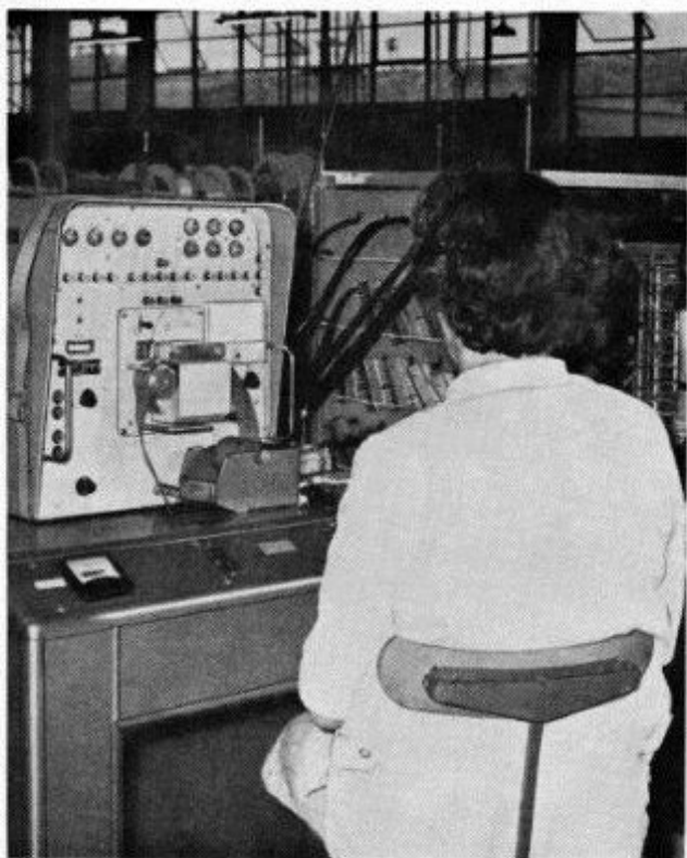
Fig. 5. CCU undergoing test on tape controlled 'Robotester'.
