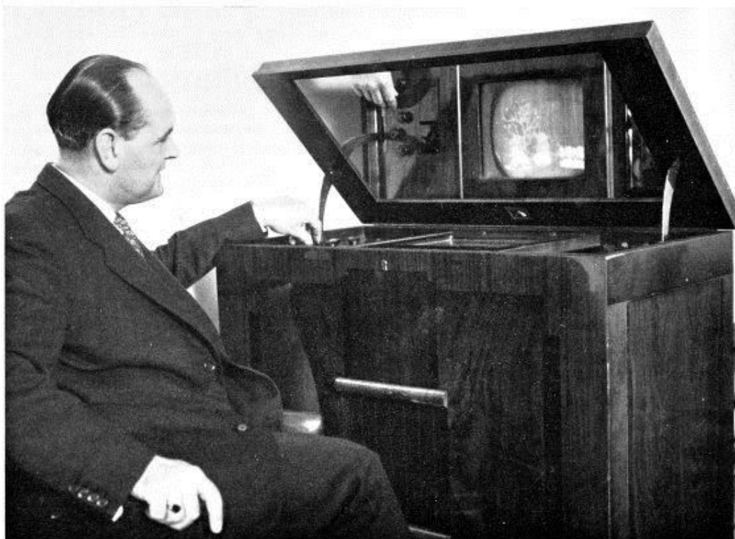
Fig.1 An HMV receiver of very advanced design in 1935 with a reflecting mirror contained in the lid of the cabinet.
