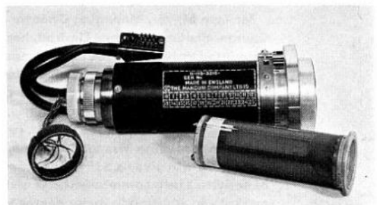
Fig.5 The Mark VIII toroidally-wound alignment coil, yoke assembly and scan coil assembly.
