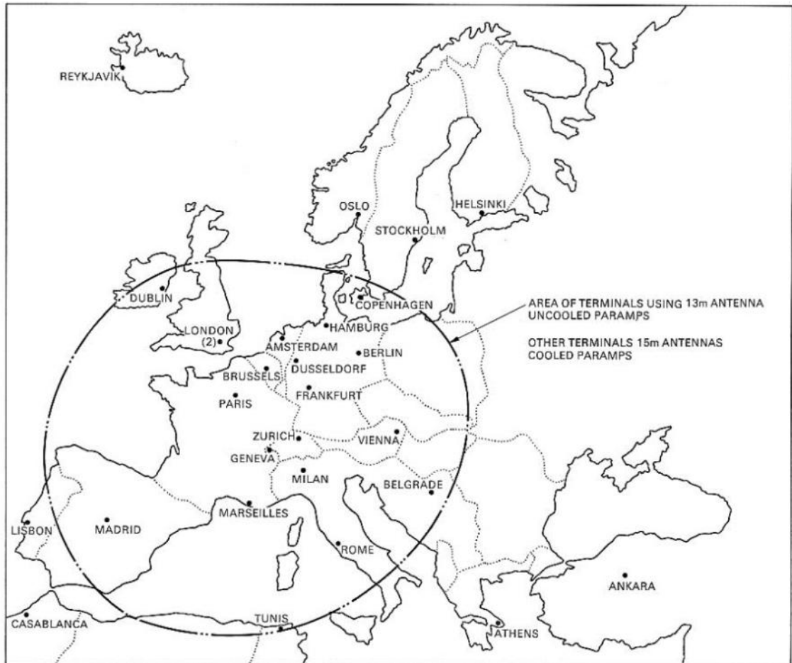
Fig.3 Estimate of ground terminals for the first phase of a Eurovision satellite network.
