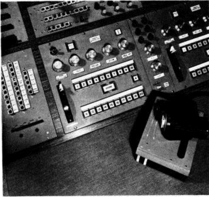
Fig.5 Main and camera control panel with multi-function hand controller.
