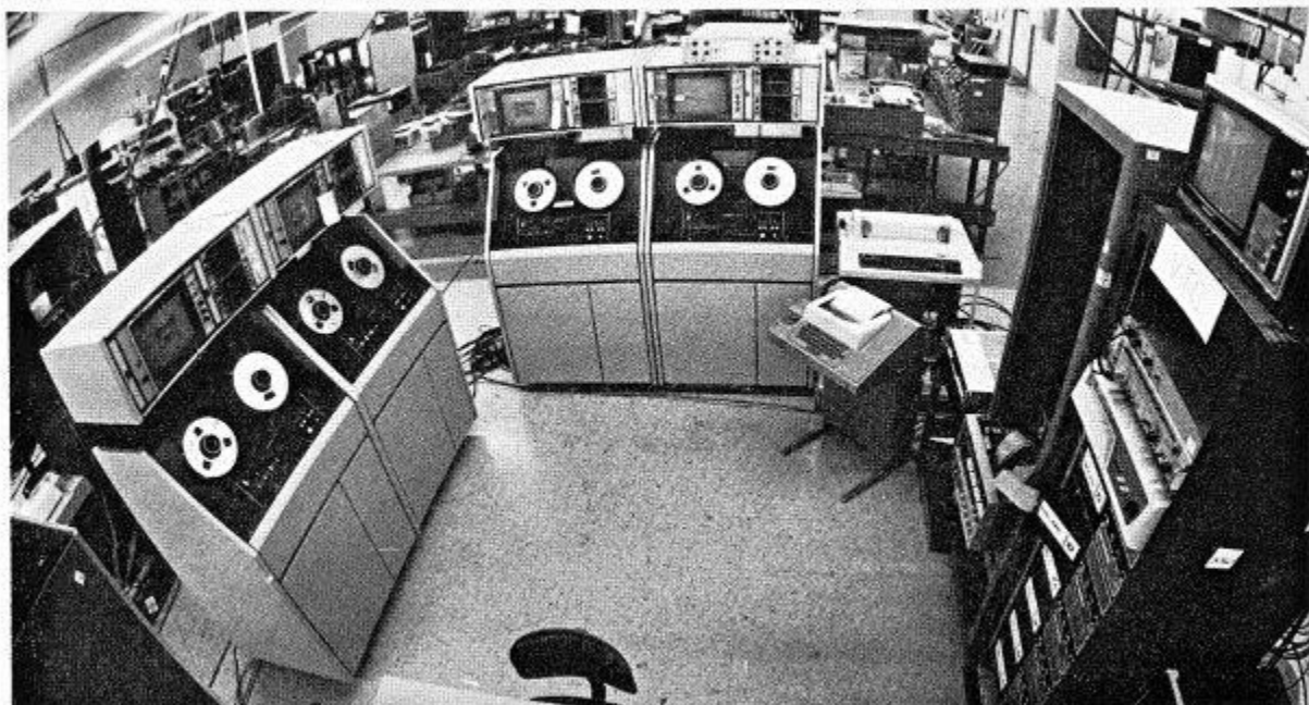
Figure 3. A CMX 340 X about to leave the Santa Clara facility. Interfaced with a modern production switcher and four VPR series one-inch helical recorders, this combination will serve as a production centre for a major TV facility
