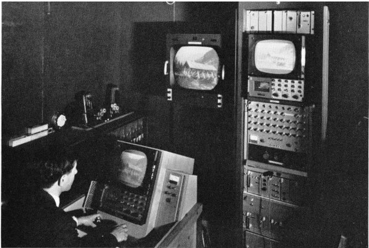
Colour film can be switched into the programme by the producer when he wants it. Here monitoring the 35 mm telecine picture is Barry Lorkin with the black-and-white picture and waveform monitor in front of him, and the transmitted colour picture above
