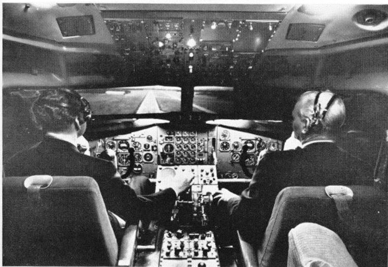
BELOW: The runway is reproduced on the screen by the projector, and the pilot makes his approach by normal flying methods
